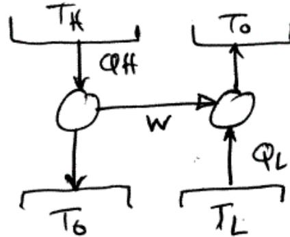
$$\frac{1 - \frac{T_0}{T_H}}{\frac{T_0}{T_L} - 1} \sqrt{\frac{T_H}{T_L}} \quad (2)$$
