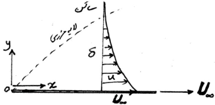
$$\frac{d}{dx} \int_0^\delta \left(1 - \frac{u}{U_\infty}\right)^2 dy \quad (2) \qquad \frac{d}{dx} \int_0^\delta \frac{u}{U_\infty} \left(1 - \frac{u}{U_\infty}\right) dy \quad (1)$$
